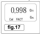
Case 2: "USER". If, on the other hand, calibrations have been made by the user, the display page will appear showing the currently used calibration factor (in our example 0,998) (fig.17).
